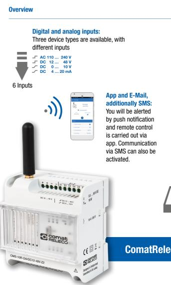
The CMS-10R is a remote monitoring and control system for industrial and building technology. It reports status changes of the digital or analogue inputs via the mobile network through push notification, e-mail or SMS. The outputs are controlled by push notification via web browser or smart app. If required, the configured outputs can also be switched with a call-in function (call to the device). The CMS-10R automatically selects the network generation with the highest field strength on site.
