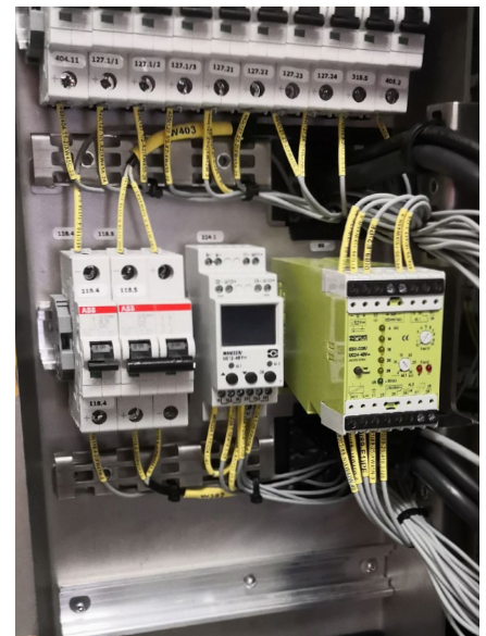
Multifunction monitoring relays secure the power supply and protect the vehicle electronics.
